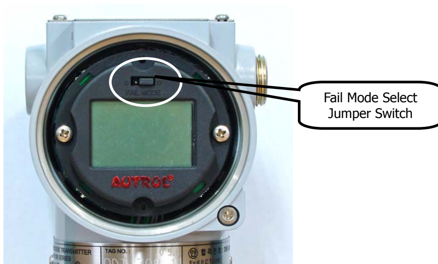
[Figure 3-2 LCD Module's Fail Mode Select Jumper]
